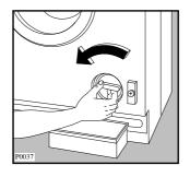
Unscrew and remove the filter.
